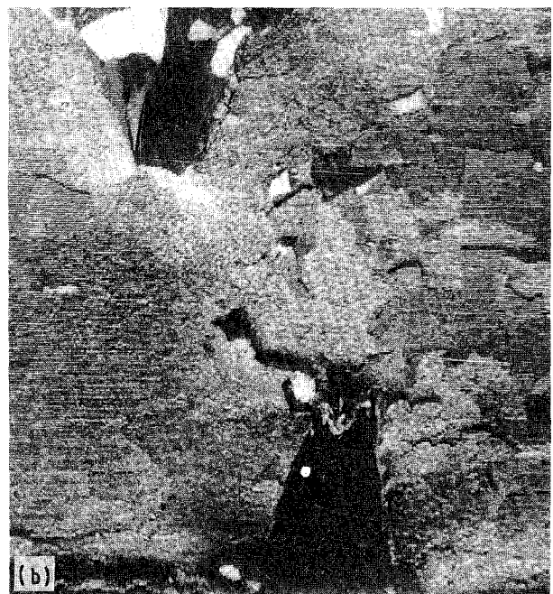
Figure 6 Scanning electron micrographs for copper plates under mixed-mode deformation, containing two staggered edge cracks.
